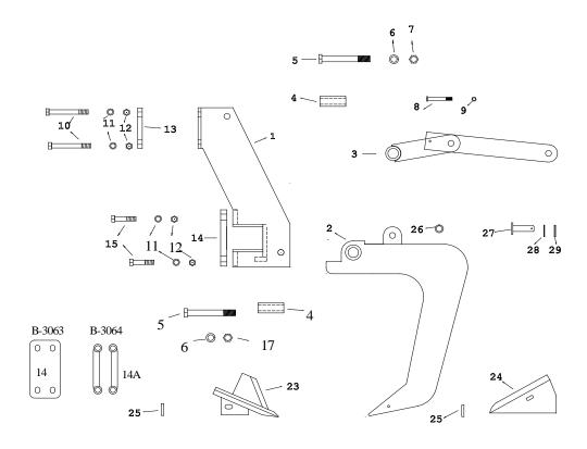
AE 1" & 1 1/4" SHEAR TRIP SHANK ASSEMBLIES: A-2508-TMT, A-2509-TMT
