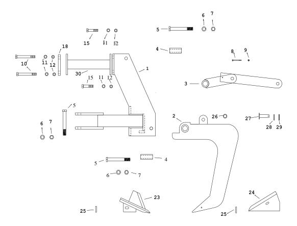
AE 1" & 1 <sup>1</sup>/<sub>4</sub>" SETBACK SHEAR TRIP SHANK ASSEMBLIES: A-2508-TMTB, A-2509-TMTB
