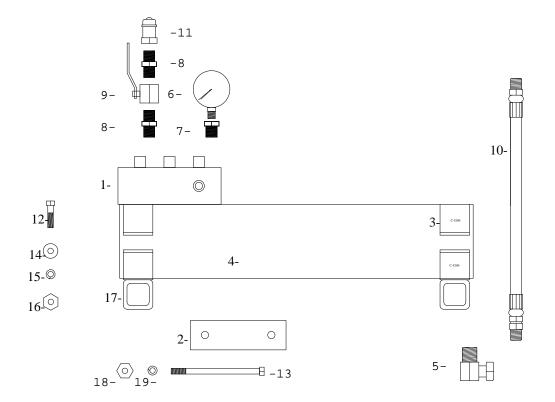
HYDRAULIC ACCUMULATOR ASSEMBLY, 1 GAL.: A-3540
