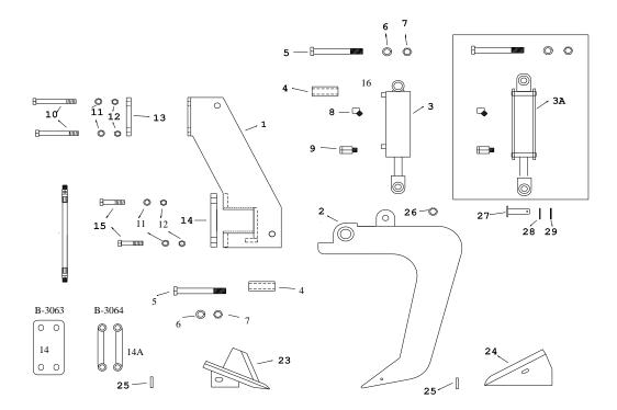
TM 1 & 1 <sup>1</sup>/<sub>4</sub>" HYD. RESET SHANK ASSEMBLIES: A-2508-TM, A-2509-TM, A-2518-TM, A-2519-TM
