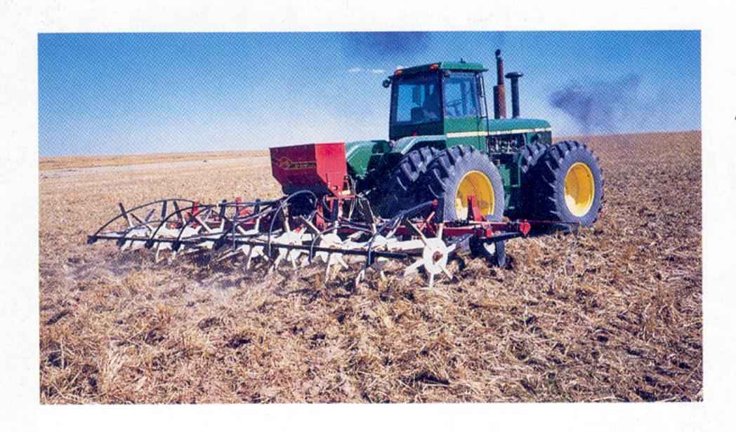
A Dammer Diker with an air seeder can be used behind conventionally planted grain. A small amount of seed is placed in the reservoirs to insure 100% stand. This process will stop water movement in the fields and improve crop production. This concept works well in CRP seeding and is probably the only proven conservation tillage machine for small grain crops.
