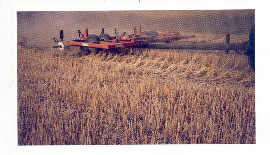
This 14 ft. pull-type *Dammer Diker* is ripping 15" deep and diking the stubble field to conserve precious moisture. These small reservoirs insure that next year's crop has maximum available soil moisture. Research shows that one additional inch of moisture can produce 7 or more bushels of grain per acre.
